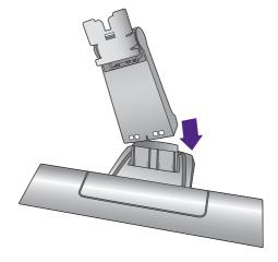
Orient and align the stand arm with the monitor, then push them together until they click and lock into place.
